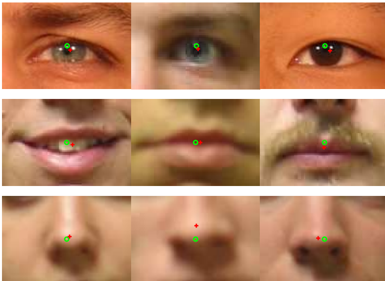
Figure 4.15: This figure provides some examples where the landmarks MLLL, BILBO and TROLL give an equal or better estimates than the manual landmarks. The green circle denotes the manual position and the red cross denotes the position found by TROLL.
